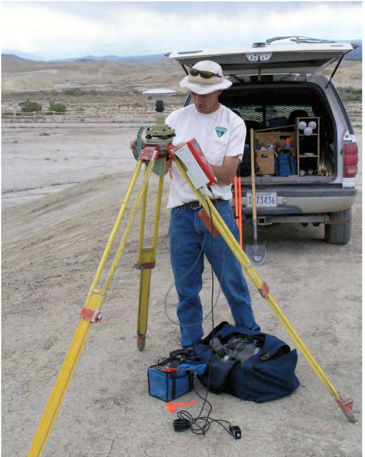
Setting up a GPS unit to reestablish positions for change detection at the Falcon Road Open OHV area within the Gunnison Gorge National Conservation Area near Montrose, Colorado.
